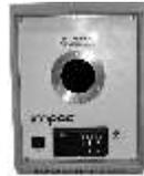
Black body furnace is also a dry bath, but used in non contact calibration. The black body furnace has been designed to provide stable and accurate temperature to enable professionals to calibrate non contact radiation pyrometer by comparison method.
