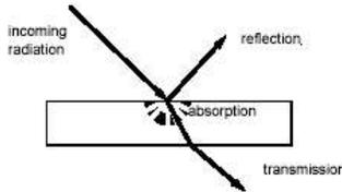
Another part of incoming rays is absorbed by dark, rough surfaces. This may happen across a wide or narrow band of the spectrum. In cinemas, much light has to be absorbed by the sidewalls of the room (often fitted out with dark
