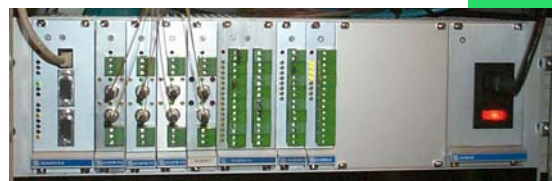
Electronic receiver, 19" rack mounted
